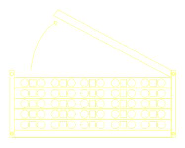
**3.**Screw the frame to the wall ensuring the frame is aligned correctly.
