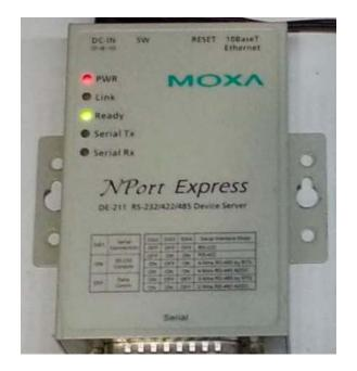
In any case, please remove the ethernet cable from the device and plug it back in, then remove the DC power jack and plug it back in to restart the device.
