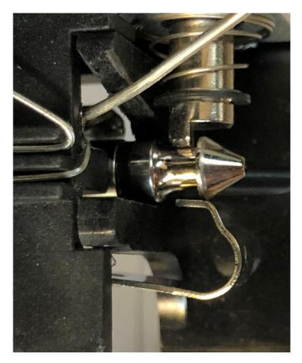
Picture above is showing a good contact between the fob and the connector.
